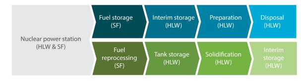
Figure 3: Generation, conditioning, storage, and disposal of SF/HLW<sup>3</sup>
